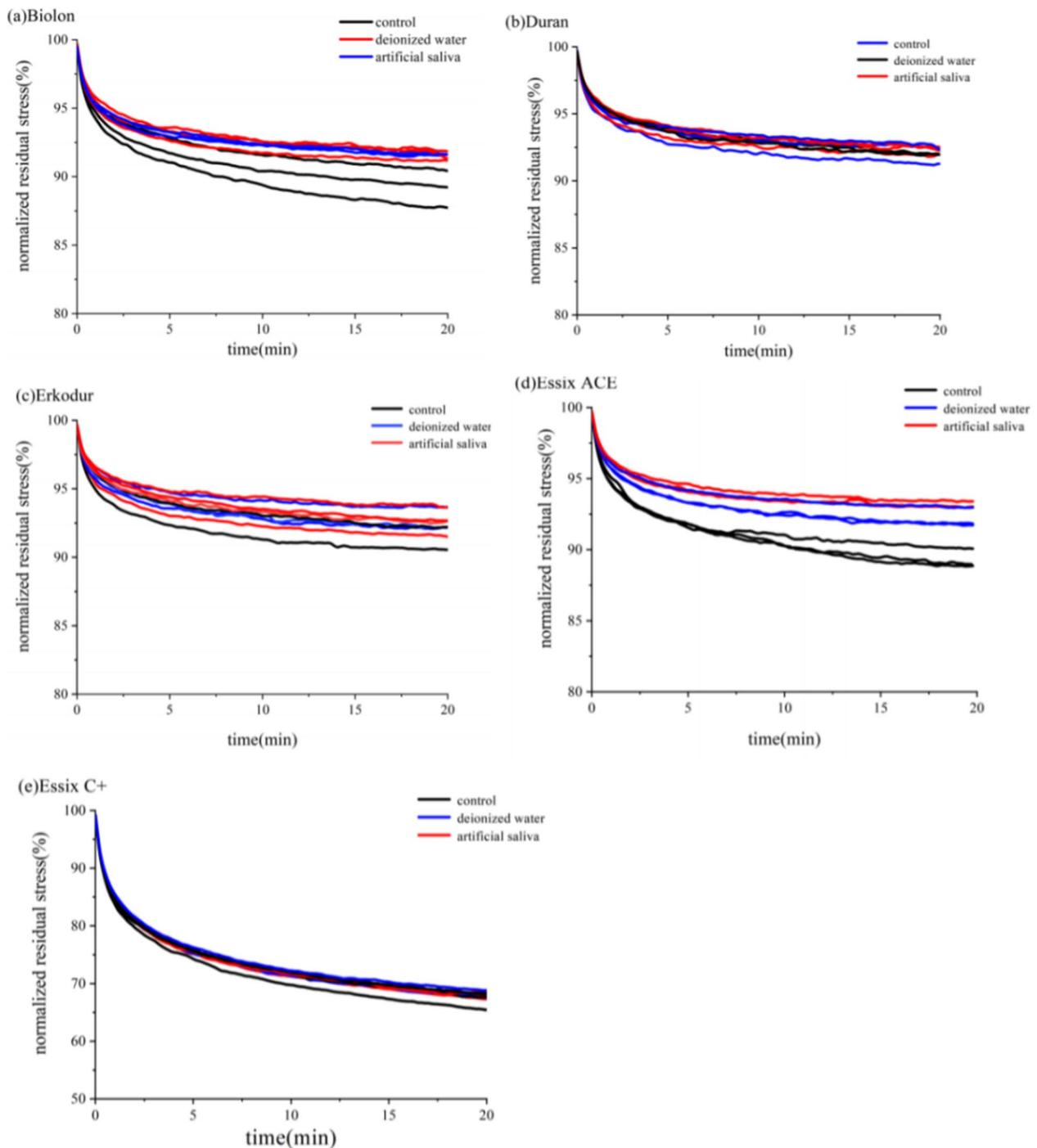
**Fig. 4** Stress relaxation curve of the five tested materials under different wet environment (a-e). Stress relaxation curve of Biolon (a). Stress relaxation curve of Duran (b). Stress relaxation curve of Erkodur (c). Stress relaxation curve of Essix ACE (d). Stress relaxation curve of Essix C+ (e)
