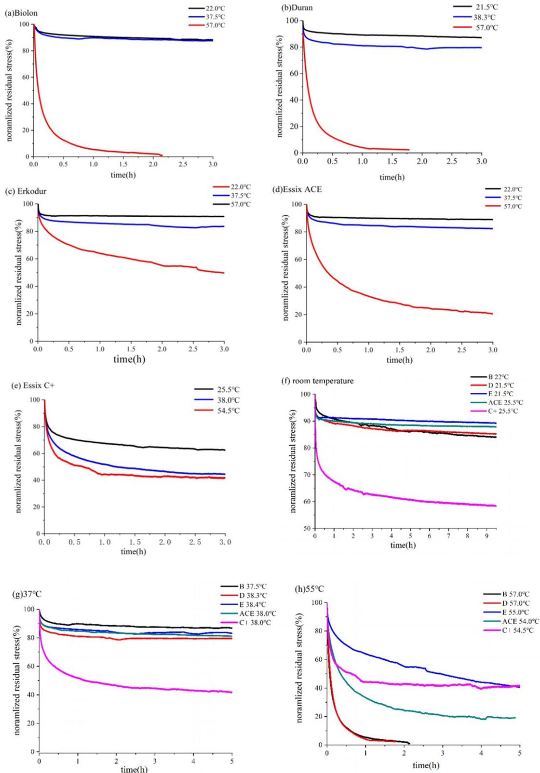
**Fig. 3** Stress relaxation curve of the five tested materials under different temperature. Stress relaxation curve of Biolon (a). Stress relaxation curve of Duran (b). Stress relaxation curve of Erkodur (c). Stress relaxation curve of Essix ACE (d). Stress relaxation curve of Essix C+ (e). Stress relaxation curve of the five materials in room temperature (f). Stress relaxation curve of the five materials at 37 °C (g). Stress relaxation curve of the five materials at 55°C (h)
