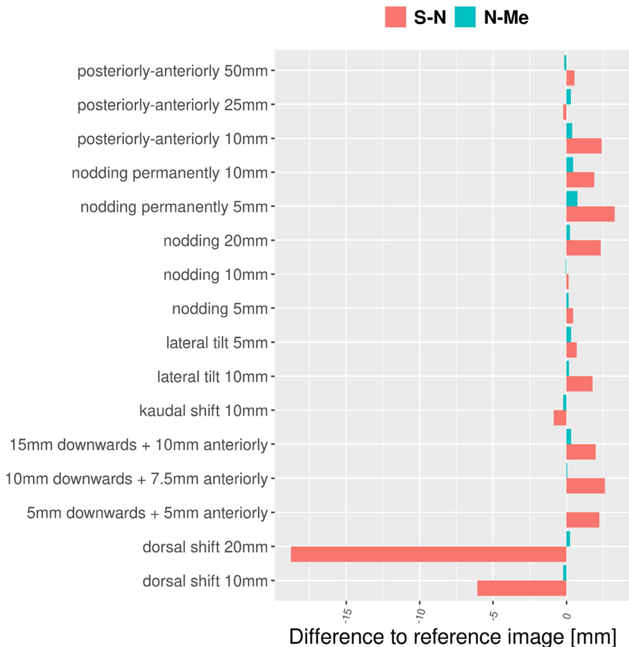
Fig. 8 Influence of motion patterns on horizontal (S–N) versus vertical (N–Me) distances
