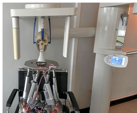
Fig. 1 Head movement simulation system with mounted dry skull prepared for x-ray acquisition
